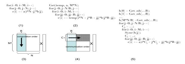
Figure 2: (1) Fine-grained loop; (2) Loop after message vectorization and cache blocking; (3) Memory order for cache blocked loop; (4) Possible memory order for packed communication; (5) Code for strip-mined loop;
