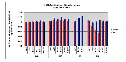
Figure 5: Results for NAS application kernels. Class A on 4 and 8 processors, Class B on 16 and 32 processors and Class C on 64 and 128 processors. Performance (Mops) is reported as relative to that of the officially released version. HAND refers to the best performing manually optimized implementation. OPT refers to the performance of compiler optimized code.
