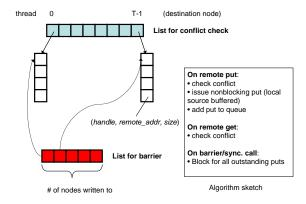
Figure 1: Runtime structure for nonblocking puts
