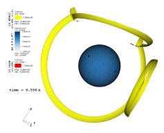
detonation front (yellow) and density on a sphere through the hot spot
