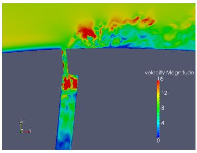
Isosurface of vertical velocity colored by velocity and cut plane through the synthetic jet (both on 3.3 Billion element mesh). *Image Courtesy: Ken Jansen*
